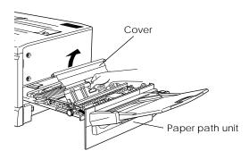
Turn the knob on the unit. The jammed paper comes out. After the jammed paper is ejected halfway, pull the paper up and out.
