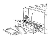
3. Take a new fuser oil roll from the box and remove the cover and two shipping pins.
