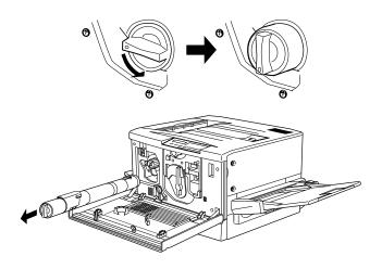
Take a new cartridge out of package and gently shake it back and forth and front to back.
