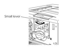
4. Pull the photoconductor unit out about 30 cm.
