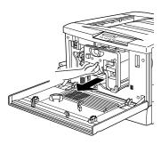
5. Grab the handle at the top of the photoconductor unit and gently pull it all the way out.
